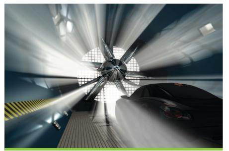
Planes, cars, bikes and many other objects are used in wind tunnels to test aerodynamics, or how an object moves through air at many speeds. For bikes and cars, we want them to be pushed lower into the ground (no lift), whereas with airplanes we want them to create lift so they can fly through the sky. Wind tunnels can be whole buildings that use powerful fans to test life size objects, or small models, like the one you will build and test today.
